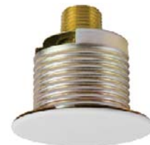
2 3/4" diameter plate STANDARD RESPONSE WHITE FLAT PLATE CONCEALED PENDENT
